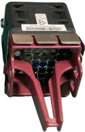
Figure 3. Cisco C9350 series field-replaceable fan unit
