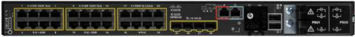
Figure 7. IE-9320-16P8U4X Switch with multi-gigabit and 4PPoE
